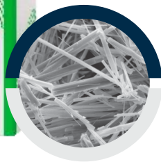
New Osteo's \alpha -hemihydrate crystalline structure
